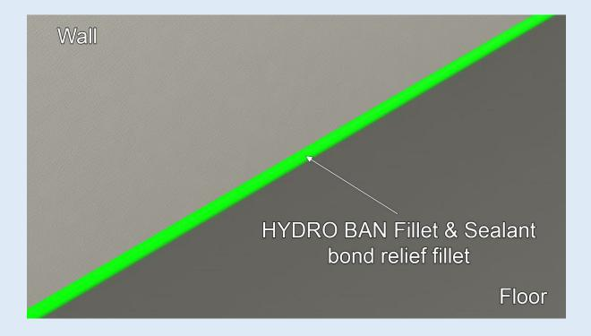
Once the area has been prepared in accordance with the manufacture's guidelines, the Bond relief fillet can be installed. HYDRO BAN Fillet & Sealant is used for this purpose.
