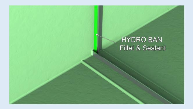
Using HYDRO BAN Fillet & Sealant, seal the front edge of the NT Wall Waterstop as shown in the diagram above, tool off any excess sealant to allow a smooth transition.
